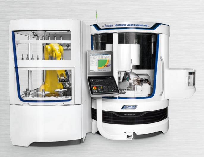
HELITRONIC VISION DIAMOND 400 L with the "Robot loader 25" (left) and "Electrode/grinding wheel changer" (right) options — the ultimate configuration for high performance
