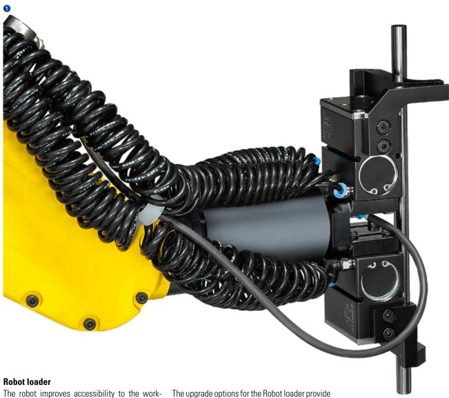
The robot improves accessibility to the workpieces and makes special applications possible. Depending on the type of workpiece or the workpiece diameter, up to 1,500 workpieces can be loaded with the standard model using the robot.
