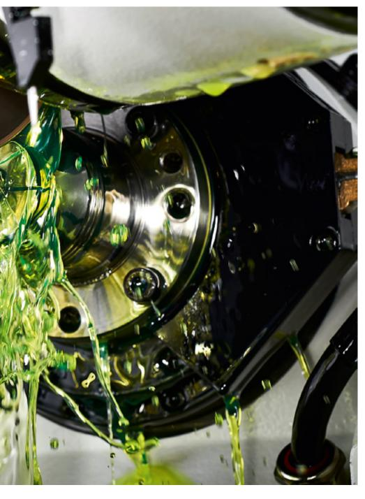
With FINE PULSE TECHNOLOGY, the HELITRONIC VISION DIAMOND 400 L sets new benchmarks for quality for PCD tools. It is an economic investment for both the production and resharpening of PCD/CBN tools in the diameter range of up to 315 mm.
