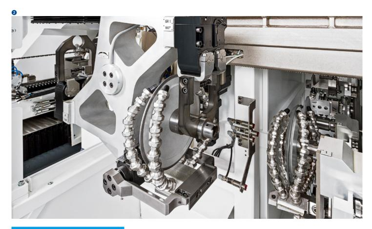
• Flexible loading systems with a capacity of up to 24 or 72 electrodes/grinding wheels
